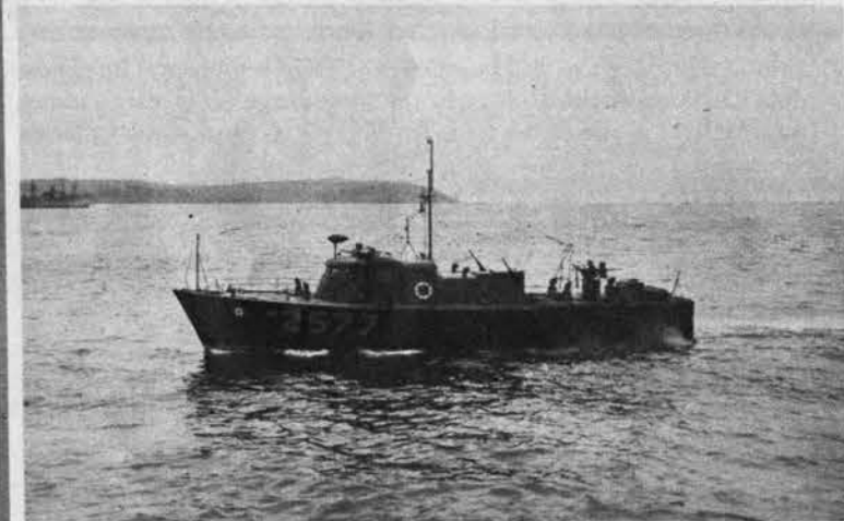
Sharp clipper bows mark most British air-sea rescue launches. This 73-ft. type has a low sturdy cabin stepped down aft, with a prominent gun mount near stern. Range is nearly 600 miles, and speed 22 knots.
